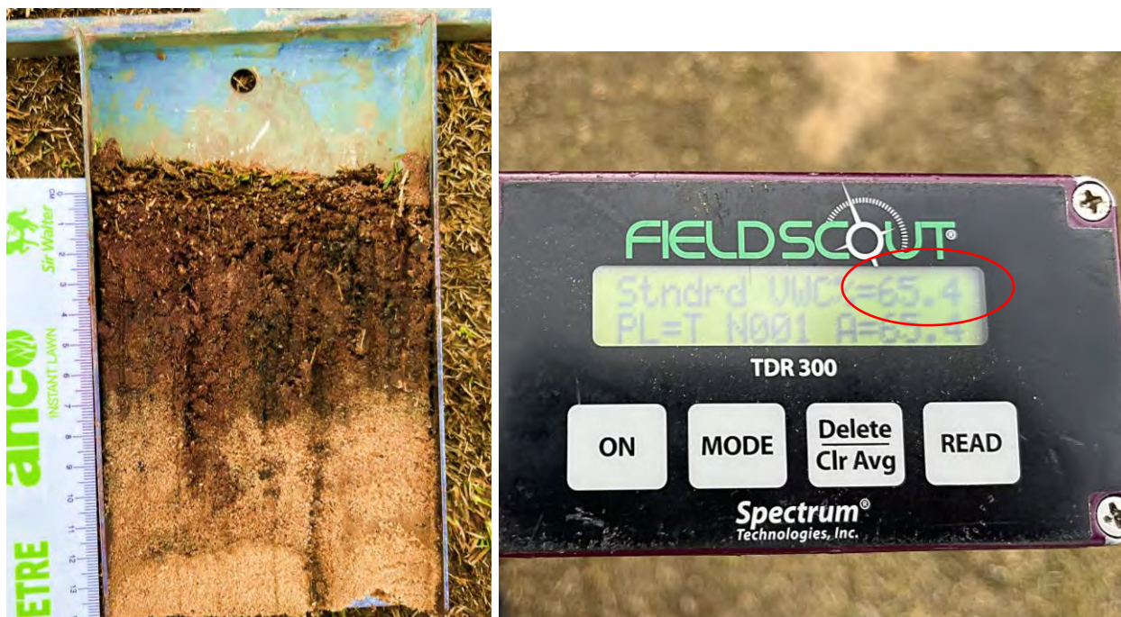
Photograph 17: Showing typical thatch layer accumulated within fairway profiles. The distinct red/brown thatch is typical of thatch derived from fescue's.
