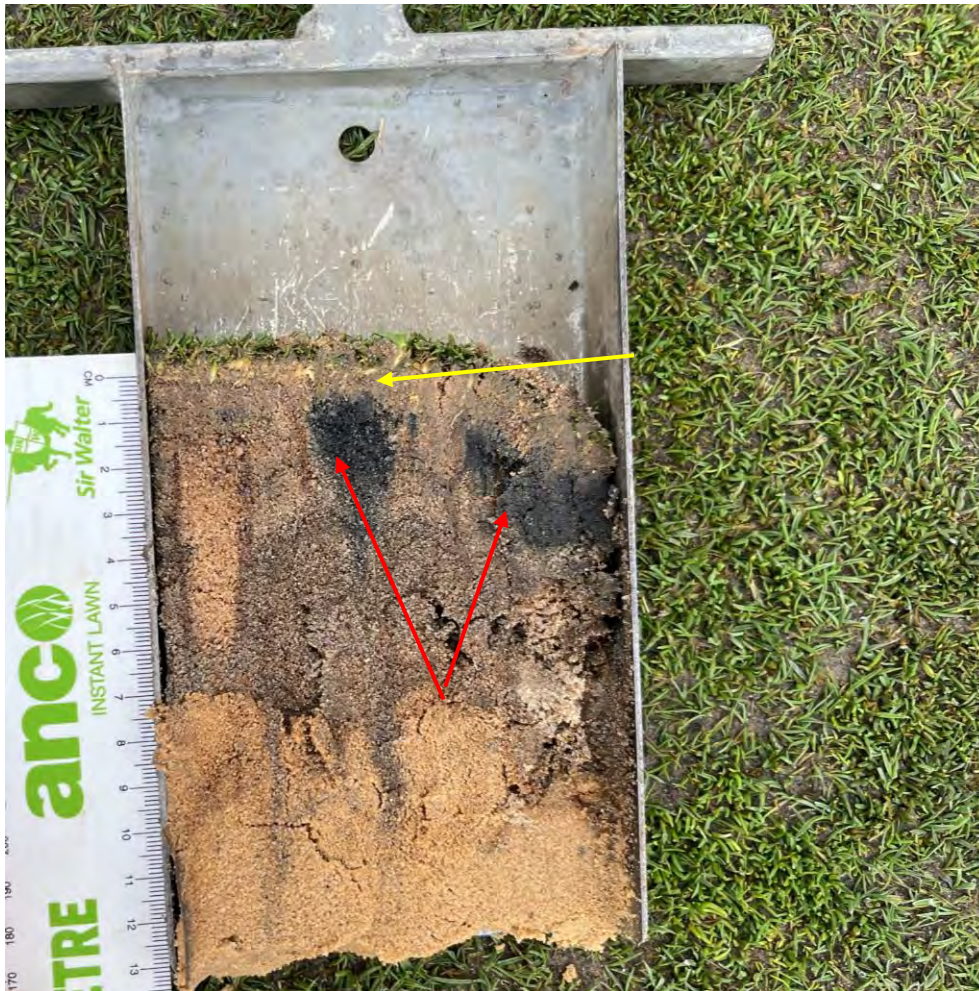
Photograph 4: showing black layer within the profile of the putting green and a distinct layer sealing the surface of the profile.
